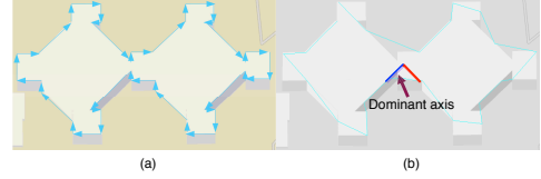
Figure 8: (a). Contour of a building (b). Two dominant axes in red and blue picked up by the contour sample in cyan
